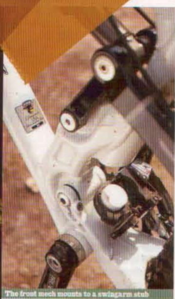
The front mech mounts to a swingarm stub
